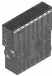
Trash box with plastic bucket, with GUGI-Ductile iron mesh grating MW 15/25 mm, black, class C 250, locked
